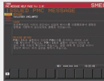
PMC alarm check function
